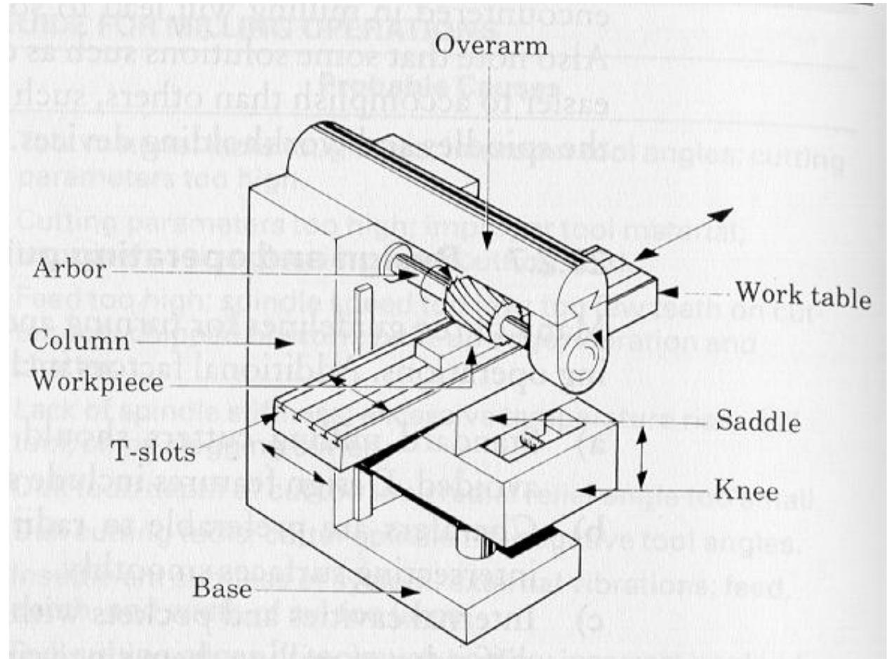
How does the table move along X- Y- and Z- axes ?
